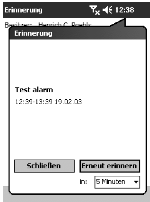
Figure 28: Alarm notification displayed on top of the power-on-protection dialog on wake up
